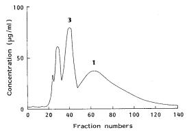
Ito's multicoil counter current chromatography. System: CHCl<sub>3</sub>-MeOH-water (7:10:8) (LP: mobil phase, UP: stationary phase). Flow rate: 4 ml/minute.
